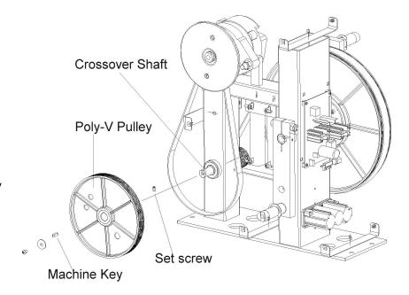
7. Install the new Poly-V Pulley in reverse order ensuring that the machine key is in place when tightening set screws.
